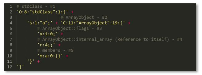
Unserializing this string triggers the bug and causes *intern*-*array* pointer in ArrayObject::unserialize to point to a slot which is freed and returned to the heap for re-allocation. However, this slot is immediately allocated (in <u>line 1798</u>) when unserializing the members array.
