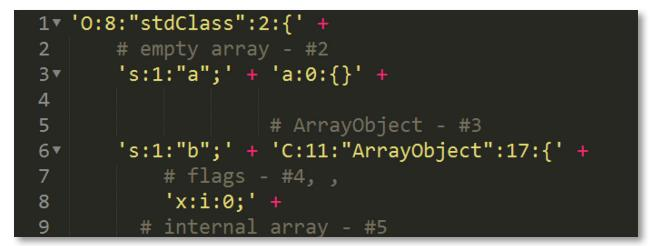
Now the internal array of the *ArrayObject* is a reference to itself (#5), triggering the bug. The members array is a reference to an empty array: the first object instantiated in the stdClass (#2). Thus, the free slot remains in the heap, and can be allocated on our terms.
