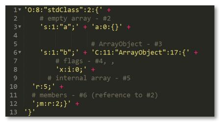
Now the internal array of the *ArrayObject* is a reference to itself (#5), triggering the bug. The members array is a reference to an empty array: the first object instantiated in the stdClass (#2). Thus, the free slot remains in the heap, and can be allocated on our terms.
