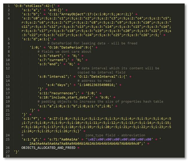
As can be seen, the offset of the *days* field in the *timelib\_rel\_time* is the same as the offset of *tz\_abbr* in *timelib\_time* struct.
