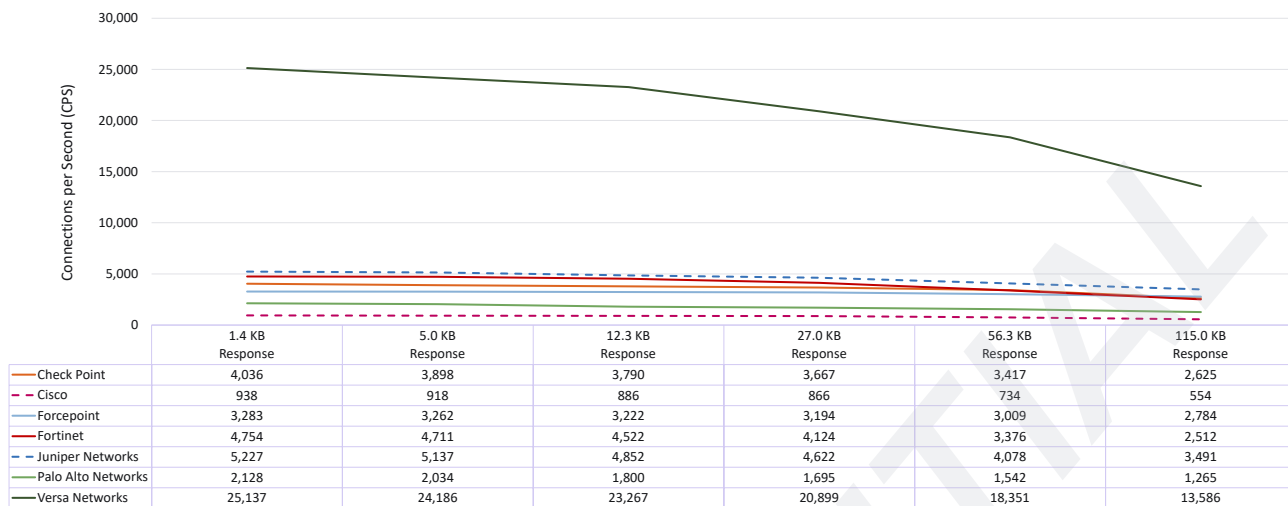
Figure 22 — HTTPS Capacity for TLS 1.3 (TLS_AES_128_GCM_SHA256 [0x13, 0x01]) (CPS)
